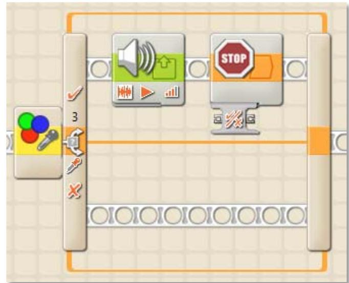
Figure 4 Switch block
